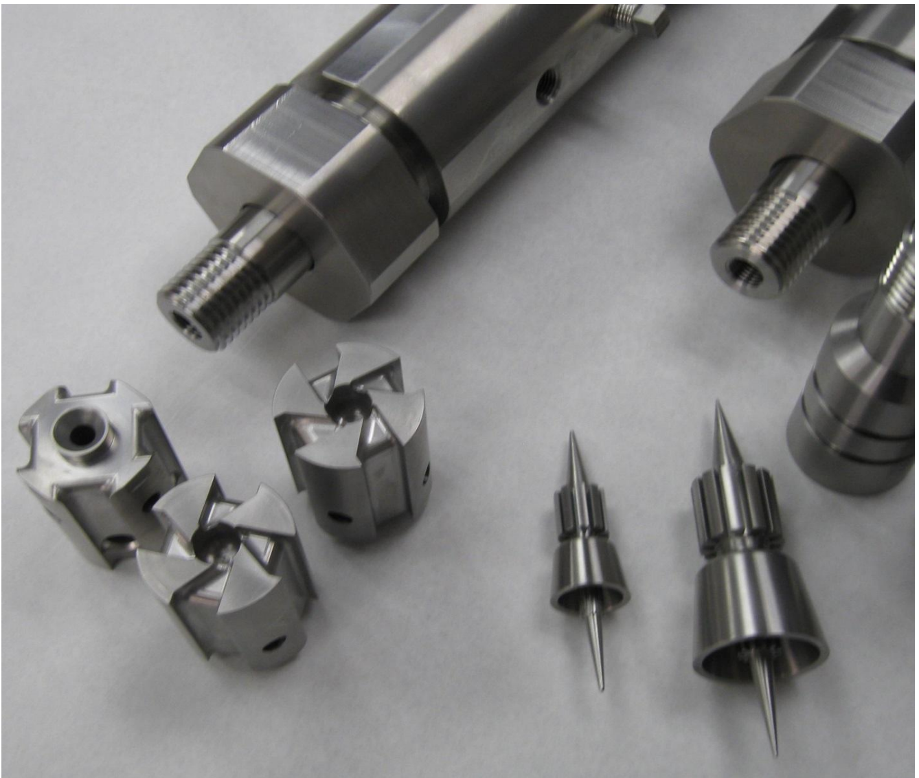
Figure 4. Geometry of the apparatus internal parts for linear three-dimensional homogenization of fluid flows in pipelines.
