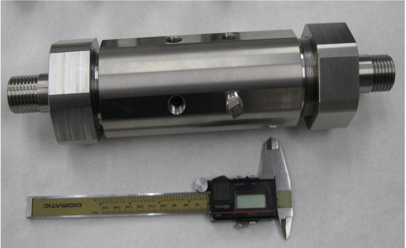
Figure 2. The scale factor of device for linear three-dimensional fluid flows homogenization in pipelines, capacity is 1000 liters per hour, if size is minimal and moving parts are completely absent.
